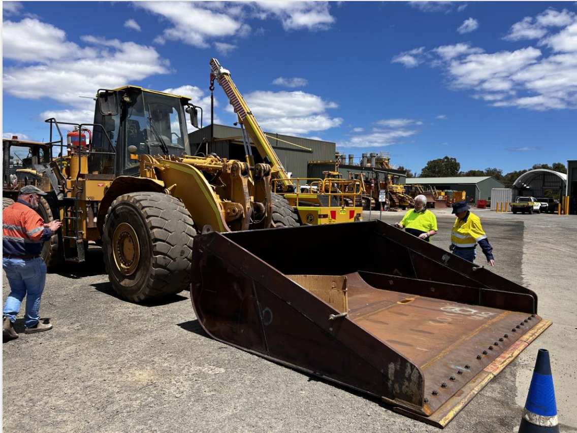
Figure 2: Modified front-end loader bucket for VDT mining method
