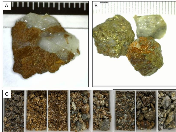
FIGURE 4: (A) RC ROCK CHIP SHOWING BROWN EUHEDRAL ANKERITE AND QUARTZ FROM CRC0012; (B) RC ROCK CHIPS SHOWING QUARTZ VEINS WITH VISIBLE CHALCOPYRITE FROM CRC0037, and (C) EACH SAMPLE REPRESENTS 1M OF RC CHIPS FROM 2M –9M DEPTH FROM CRC0037. NOTE THE HIGHLY OXIDIZED AND SULPHIDE RICH MATERIAL AS WELL AS ABUNDANT QUART.
