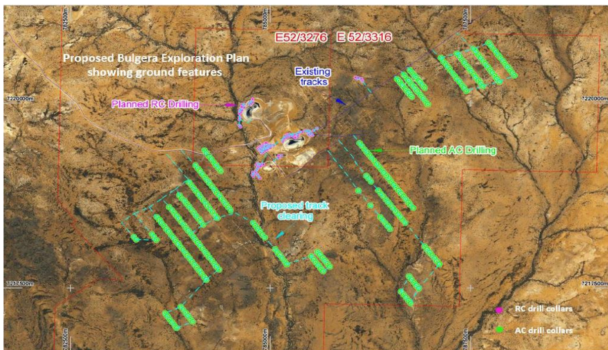
Figure 3 – Planned / cleared for hole collars for drilling to delineate near-mine surface oxide (green) and deeper (purple) gold mineralisation.
