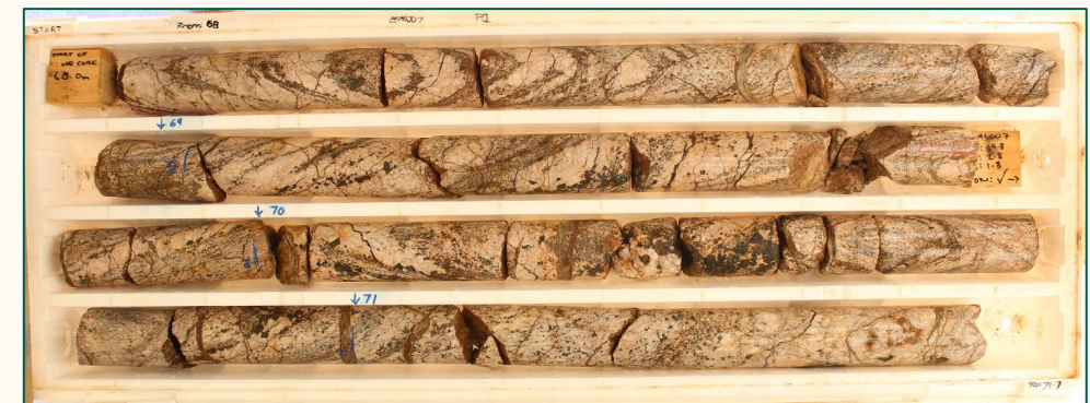
Crean - EAL007 Niobium-REE carbonatite 68-71.7m (part of 18.7m @ 1.0% Nb 2 O 5 from 65m)
