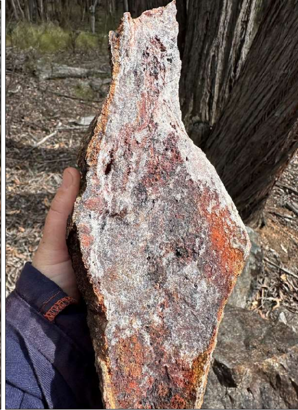
Figure 7 – Silver-Base Metal mineralisation within large baritic boulder yielding 96.7g/t Ag, 0.25% Ba 3000292
