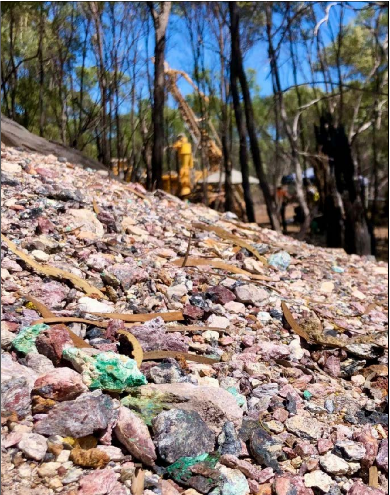
Figure 6. View of RC drill rig over spoils pile adjacent to the Sapidinus Shaft. Green malachite (copper carbonate) 3 can be seen within the pile amongst weathered pumice breccia).
