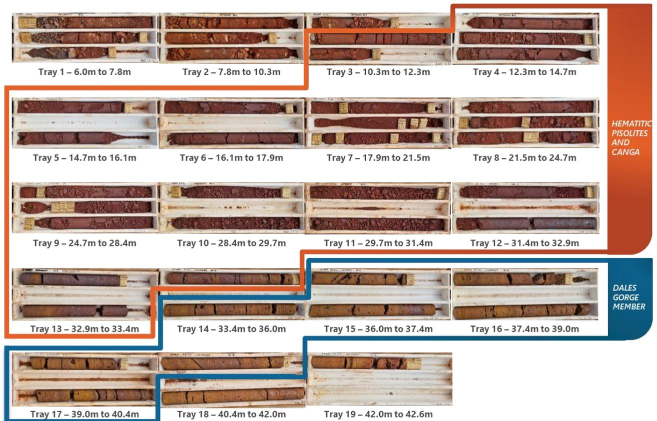
**Figure 2: Diamond drill hole METDD0171 highlighting hematitic loose and pisolitic detritals, canga and Dales Gorge Member**
