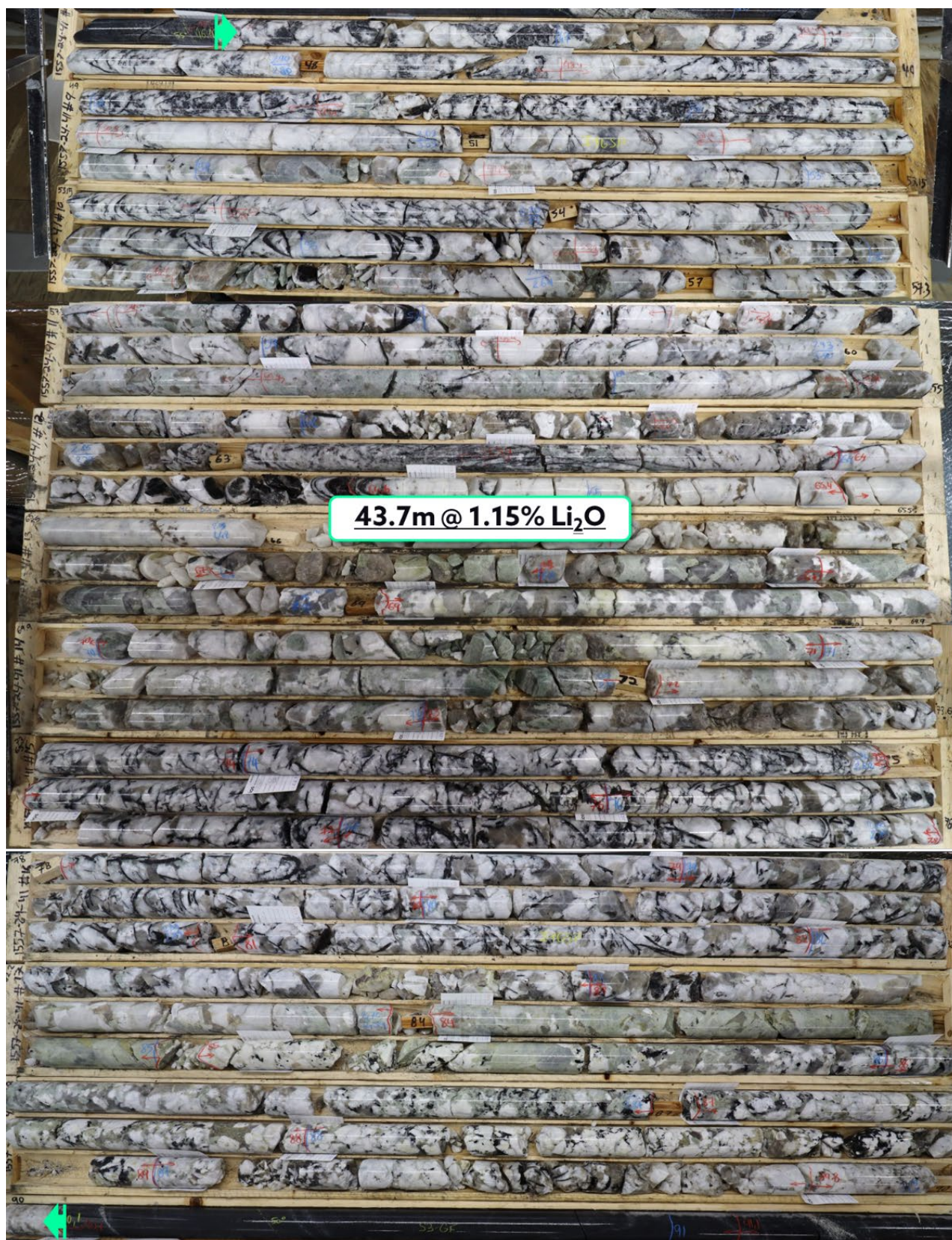
Figure 3: 43.7m @ 1.15% Li 2 O from 46.4m, including 4m @ 3.0% Li 2 O which includes 1m @ 5.9% Li 2 O in diamond drillhole 1557-24-041. 2
