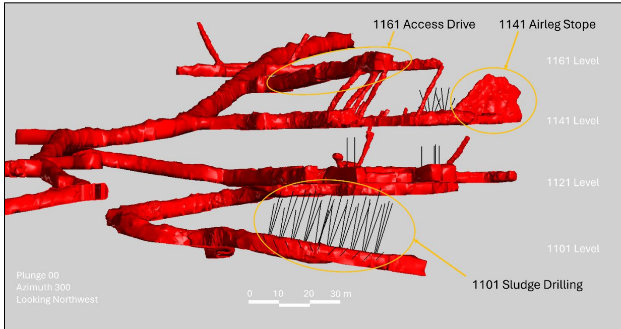
Figure 4. Zone 2 mine development and sludge drilling. Sludge drilling on the 1101 level is complete and is ongoing on the 1121 and 1141 levels. Longhole drilling is scheduled to begin on the 1101 level in late April.
