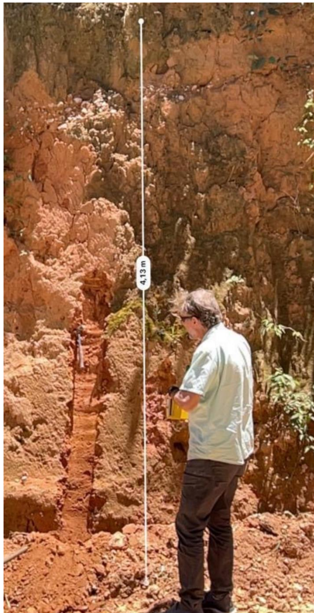
Figure 2: Examples of channel sample locations showing prospective saprolite (clay-rich zone)
