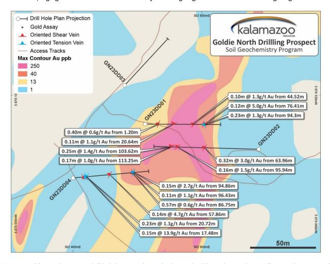
**Figure 4:** Goldie North Prospect drill hole location plan on background gold in soil anomalism. Drill traces show oriented structures and associated gold grades for results > 1g/t Au<sup>8</sup>
