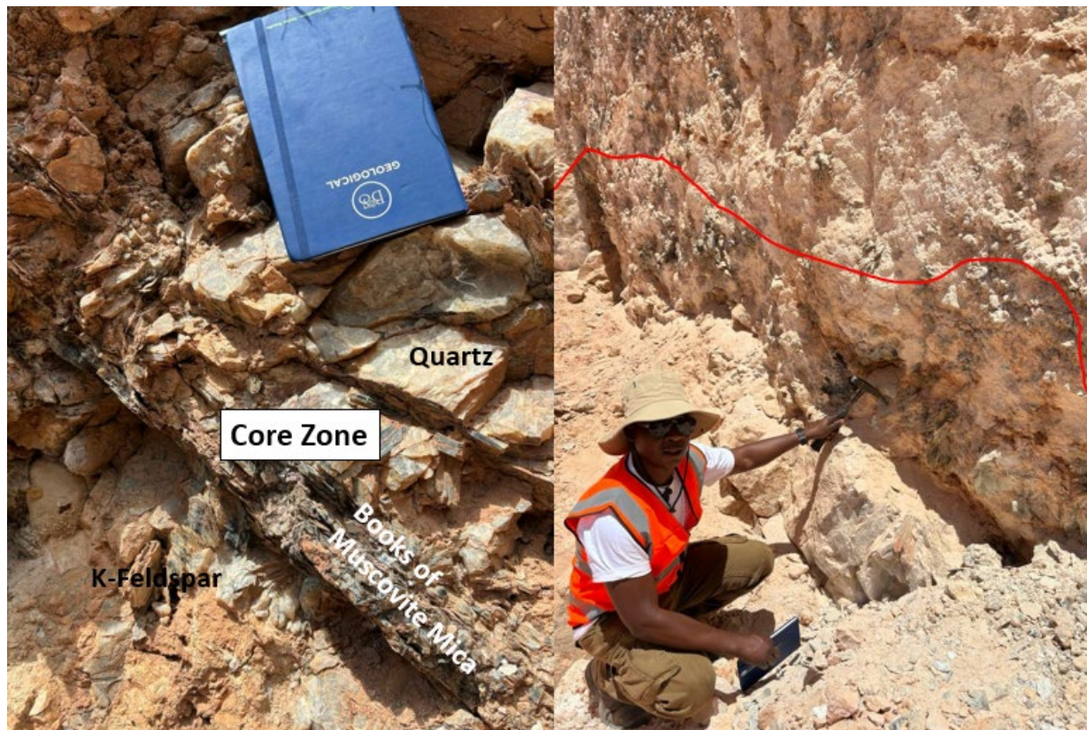
Figure 7. Core of the opened pegmatite showing quartz crystals, books of muscovite micas and K-feldspar with matrix of albite feldspar
