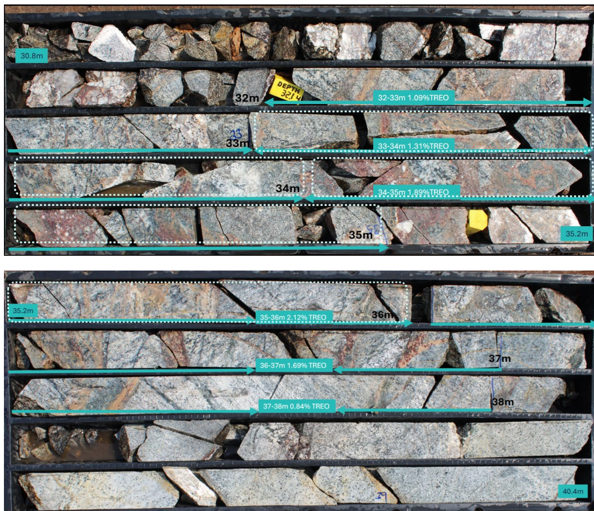
Figure 4. Half drill core of MMD007 (30.8m - 35.2m) and (35.2m - 40.4m) showing high-grade rare earth mineralisation in the Machinga deposit and pieces selected for QEMSCAN
