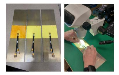
Coupons ready for testing by Boeing (L)  $CVM^{TM}$  Sensors being prepared in the laboratory for installation and testing (R)
