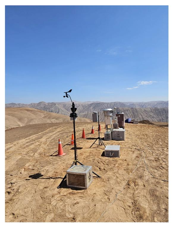
Figure 7; Environmental monitoring station at IIo Este; April 2024. For drill permitting purposes, this station will remain operational for 24 hours a day for one month.
