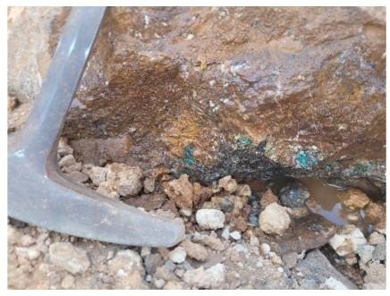
Figure 4; Copper oxides<sup>1</sup> in structures associated with calcic, sodic, and epidote alteration with specularite veining – western IOCG zone, Chancho al Palo (Coordinates 254478E, 8068009N).
