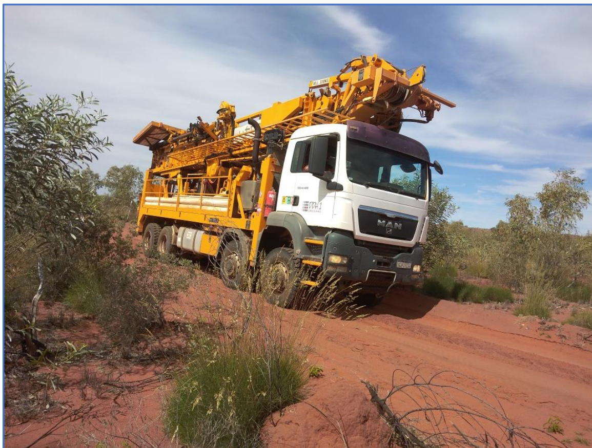
Figure 1. DDH1 diamond drill rig at Surus Site
