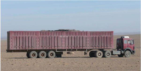
Figure 2. An example of a slow, unsafe, and dirty 'heavy duty' truck used in the South Gobi for coal transportation.
