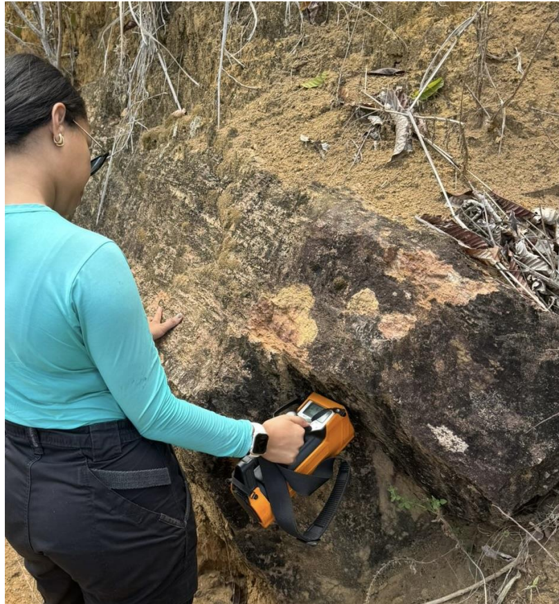
Figure 6: BRE geophysics team conducting gamma spectrometry on hard rock outcrops (Site 2) at the Sulista Project
