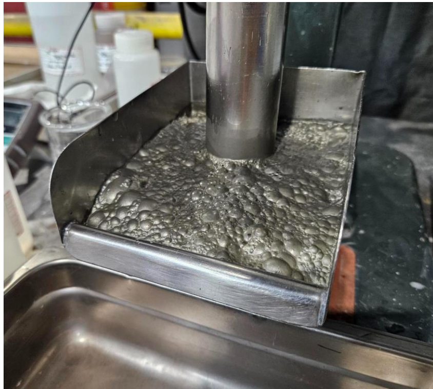
Figure 1: 3rd cleaner sulphide concentrate assaying 29.1% nickel
