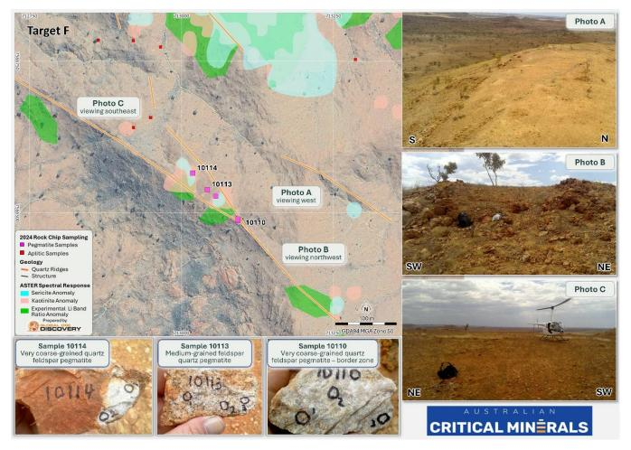
Figure 3 – Silica rich pegmatite ridges forming the lateral extents of a weathered subdued topographic low representing the inner zone of the pegmatite intrusion.
