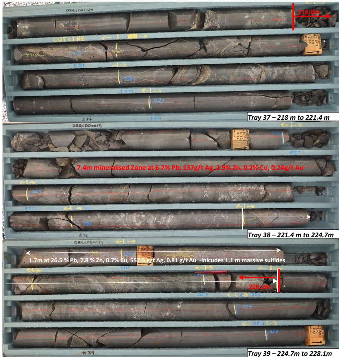
Figure 5 – Base Metals Mineralised Zone DRRCD0019. Refer Table 1 for Mineral abundance estimates.
