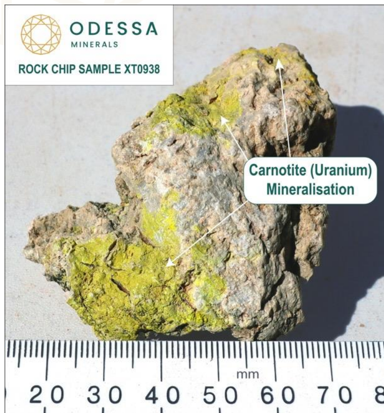
Figure 12: Carnotite (uranium) mineralisation within siliceous calcrete at the Jailor Bore prospect in Odessa sample XT0938.
