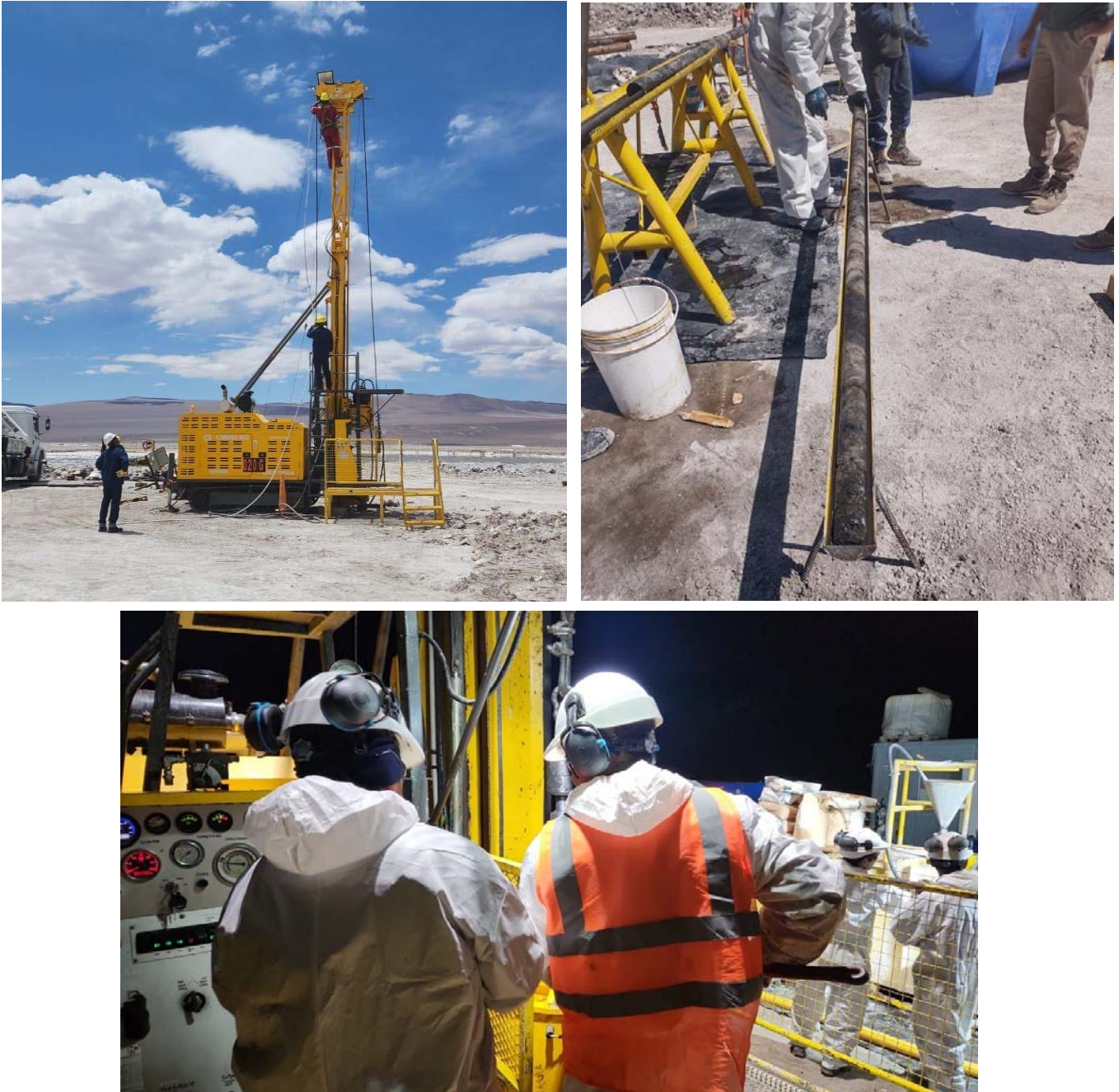
Figure 4: Drilling and core retrieval from DDH-1 at the Rio Grande Sur Project
