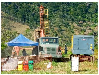
Figure 6: RC drill rig drilling at the Rio Negro prospect.
