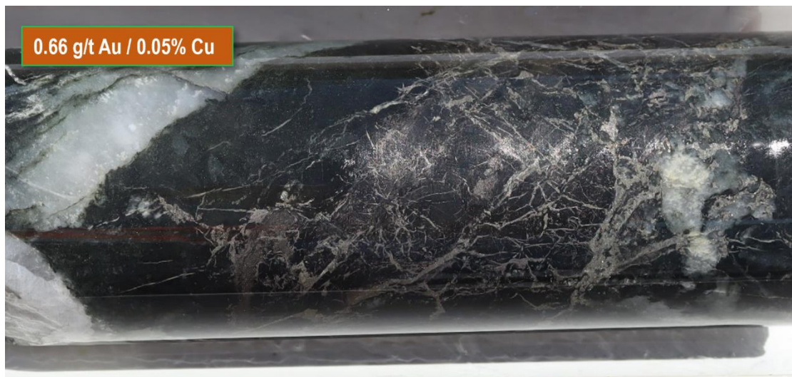
Figure 4: Mineralised Larramore core from hole 23LMDD010 (83.98-84.30m core interval) within an assayed sample length of 83.5 to 84.04 (0.54m) returning 0.66 g/t Au and 507 ppm Cu.
