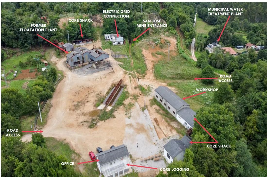
**Figure 8.** Ground view of San Jose Mine Site & Facilities (looking North)
