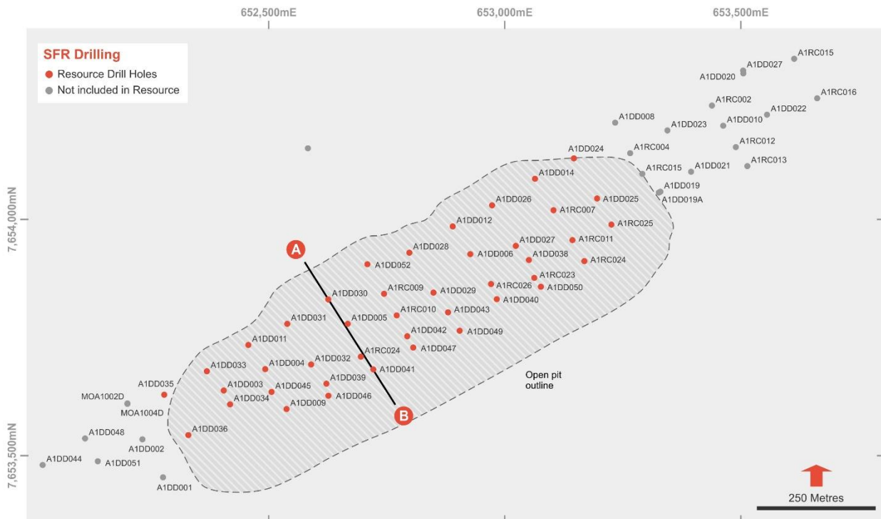
Figure 2: A1 Drill Collars included in the Mineral Resource. See Figure 3 for Section A-B.
