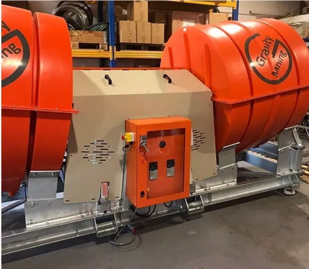
Figure 3 A Multi-gravity Separator (MGS)
