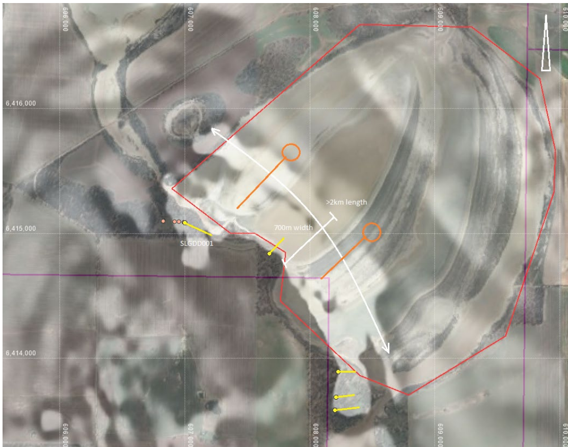
Figure 3: Plan view of 1VD magnetic signature representing the >2km long, 700m wide ultramafic sequence overlain by aerial photography highlighting the salt lake, with Reserve 18455 (Lot 225568) highlighted in red. Sultan’s 2022 aircore collars are marked in orange, and previous diamond drilling traces in yellow, with recent SLGDD001 named. Orange circles and traces indicate possible drilling collar positions to test the layered intrusion from the salt lake surface.
