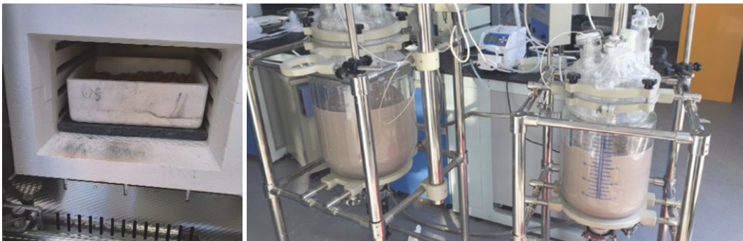
Sulphation Roasting (Left) and Leaching (Right)
