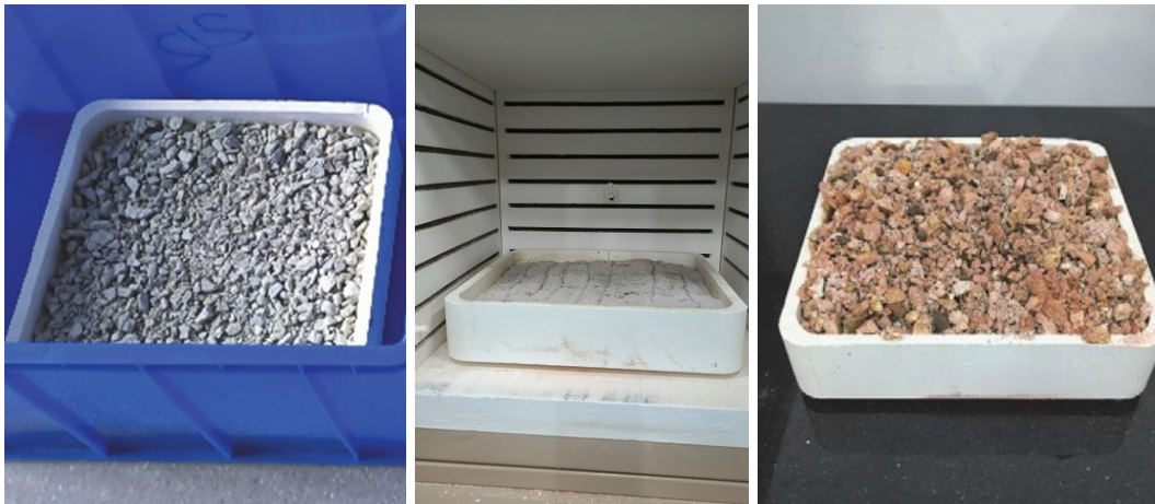
Calcination of Spodumene – Before and After
