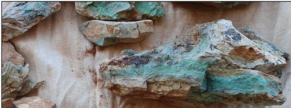
Photo 2. Rock chip sample KB03113, which returned 15.3% Copper 5 , comprised of oxidized white meta-tuffaceous siltstone with oxide copper mineralisation (green/dark grey in photo).
