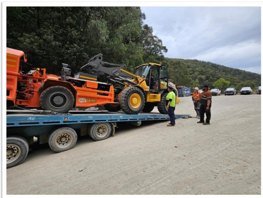
Figure 2: Volvo IT hole charger and remote controlled LHD being deliver to the mine site representing the full fleet required for increasing production
