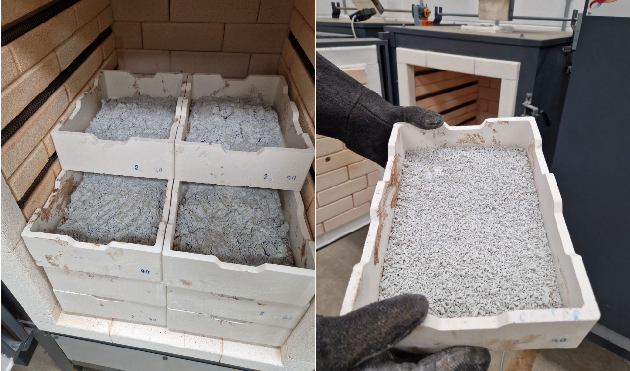
Figure 3: First NdPr oxide (>99.8% grade) production achieved from continuous operations at Ionic Technologies' Belfast Demonstration Plant.
