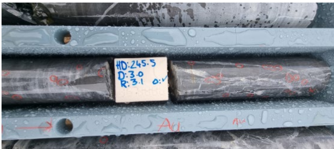
Figure 4 BKC015 Abundant visible gold (inside red circles) within a quartz-carbonate breccia hosted in metasediment
