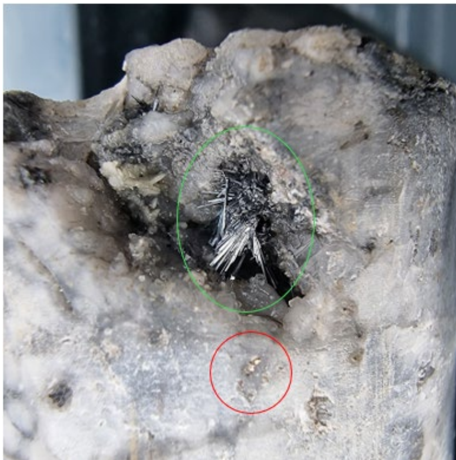
Figure 3 Acicular needle stibnite growths (green) in a late-stage vug in one of the quartz-carbonate breccias which also shows a cluster of native gold grains (red circle) just below the vug. (BKC015)
