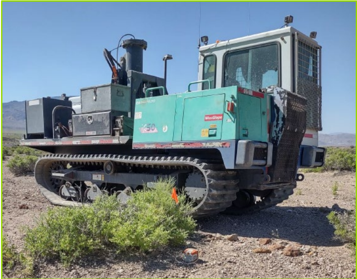
Figure 6: Accelerated weight drop seismic survey source.
