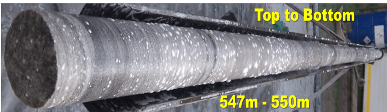
Figure 8. Three metre core run from 547-550m with gassy sandstone below coal zones.
