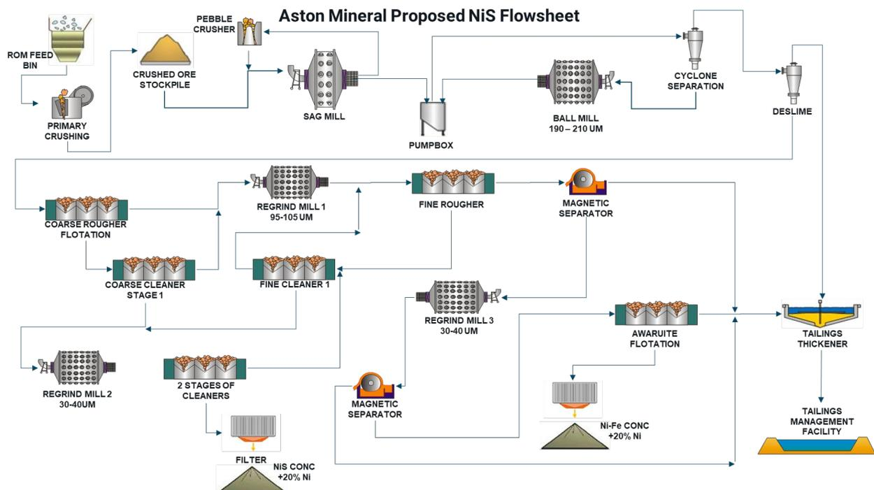
Figure 10: Simplified metallurgical flowsheet
