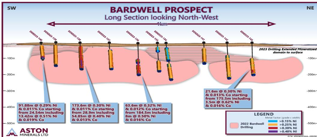
Figure 6: Long-Section Short-Hole Drilling at the Bardwell Zone
