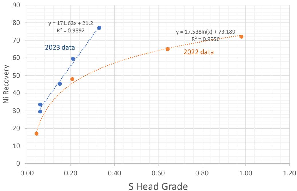
**Figure 8: 2023 recoveries from rougher flotation compared to 2022 test work as a function of sulphur head grade**
