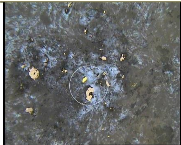
136001.10. Free gold along with bismuthinite, arsenopyrite and pyrite interstitial to wollastonite altered to carbonate. 600µm. ppl/rl.
