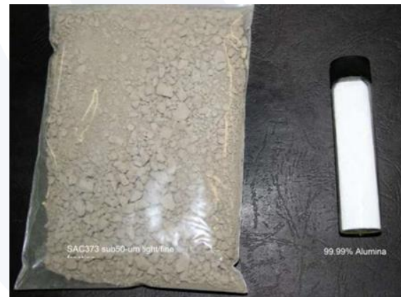
Above: Saprolitic clay from SAC373 used to produce HPA via testwork by Salazar Gold
