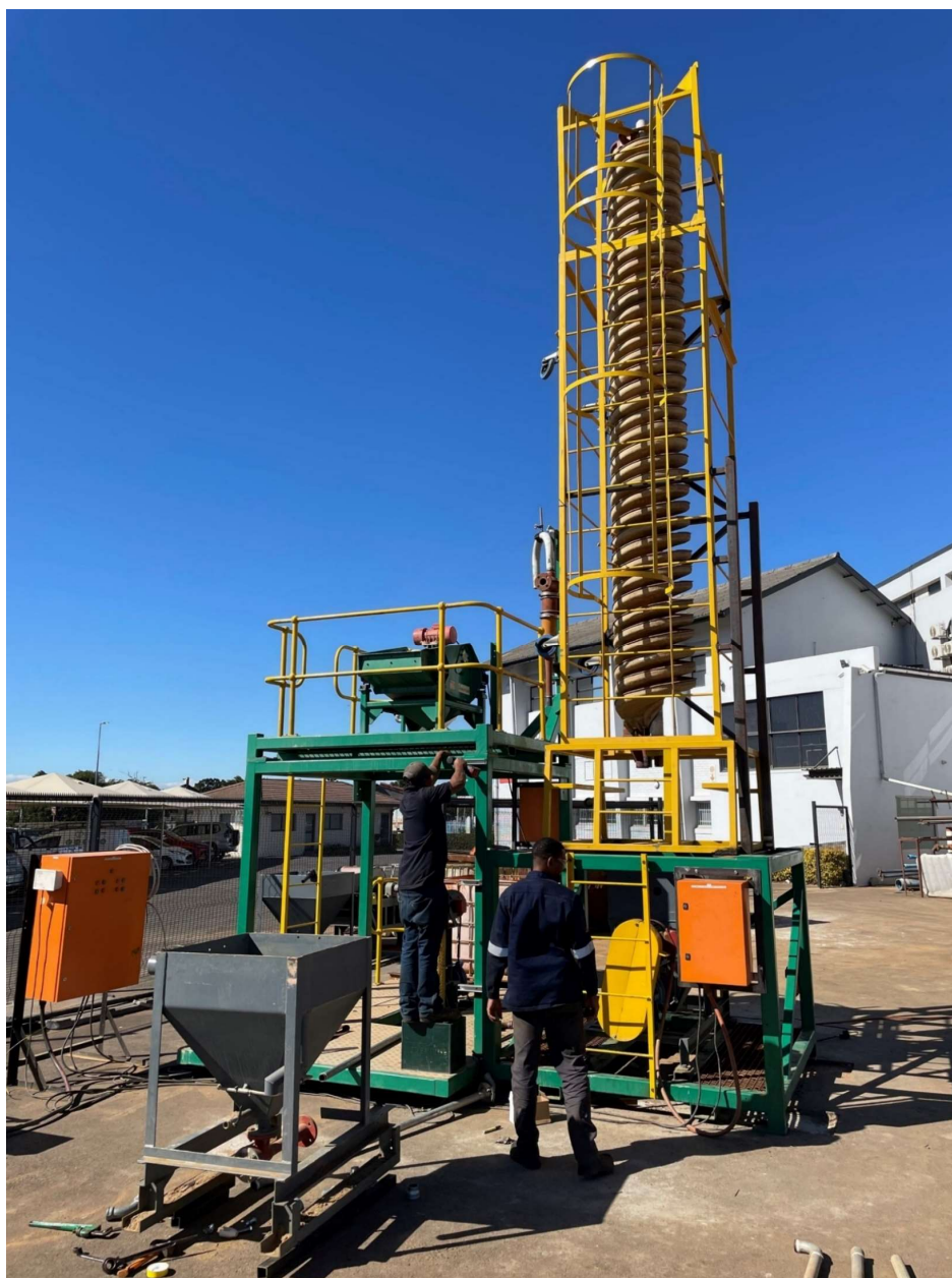
Figure 1: Final stages of assembling the spiral plant at Paterson & Cooke, South Africa
