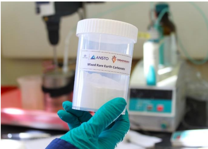
Figure 1: Photo of the high quality MREC produced by ANSTO using a conventional low-temperature acid bake/leach process.
