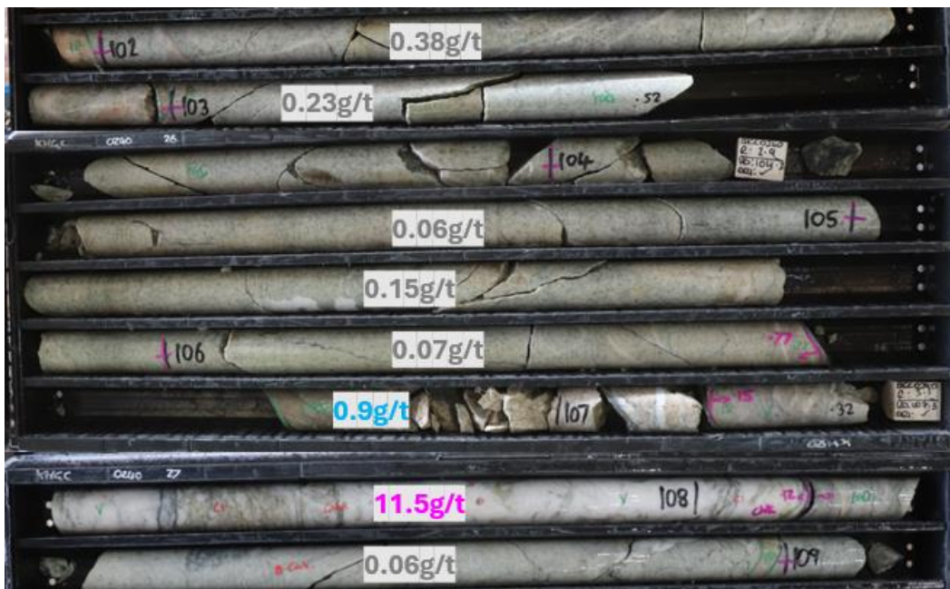
Figure 4. KHGC0240 showing mineralised section from 102.0 to 108.1 metres which graded 6.1m at 2.0g/t. Key structure from 107.1 to 108.1 metres grading at 11.5g/t.
