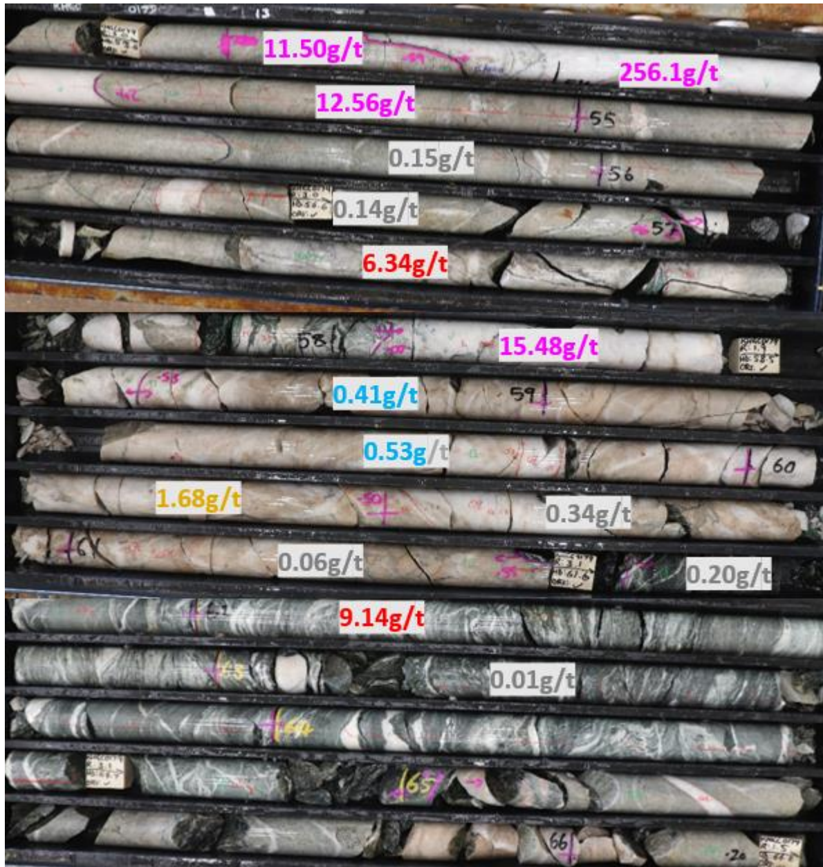
Figure 7. KHGC0179 drilling through the granodiorite and ultramafic contact below active mining fronts. 10m at 17.9g/t from 53m, within a wider zone of 25.5m at 7.3g/t.
