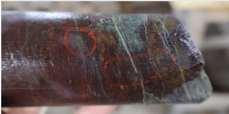
GC24-04: Close-up of uranium mineralization in core sample with peak radioactivity (8,662 cps) at 107.87 m
