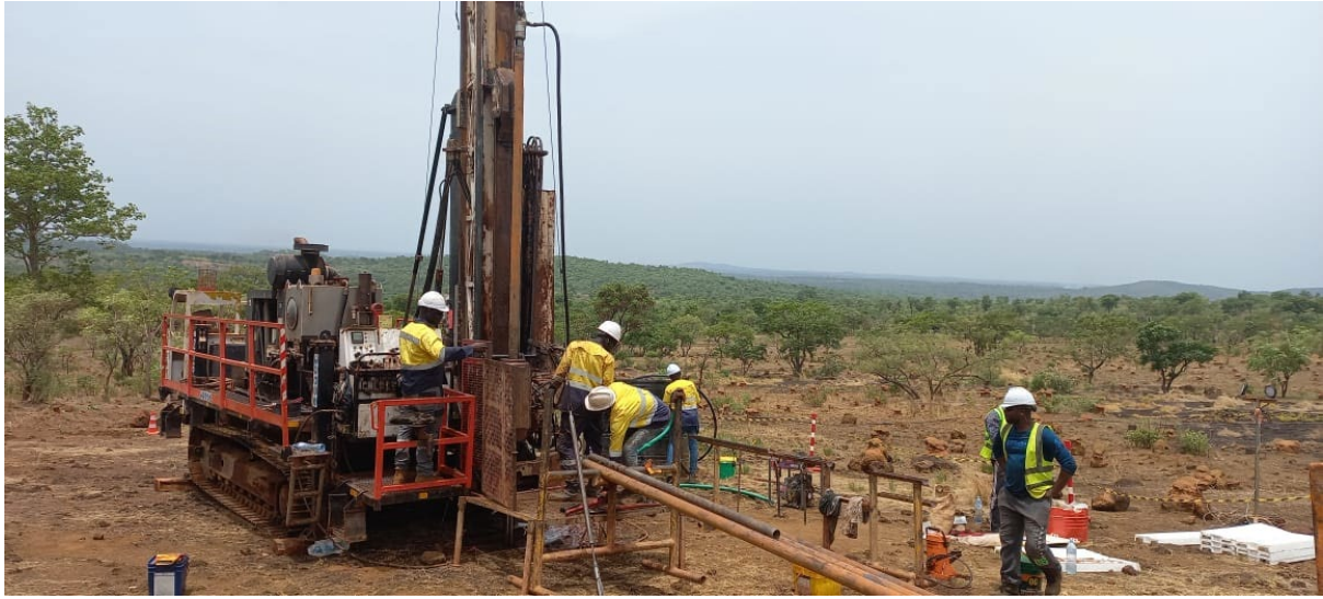
Figure 12: Guinee Forage LF-90 core rig drilling canga at Kalako target, 4 May 2024
