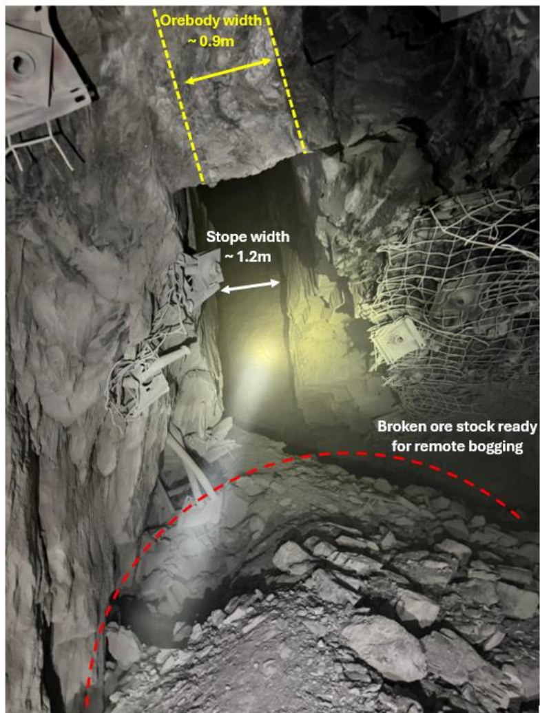
Figure 2 - Long hole open stoping at Second Fortune. Looking south on the 1085 Level Main Lode (April 2024) Highlighting narrow stope width, clean extraction with limited dilution and good ground conditions
