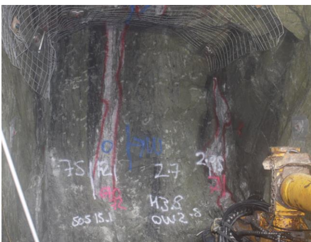
Figure 6 - 1085 Main Lode North - Cut 21 (Split fired cut)
