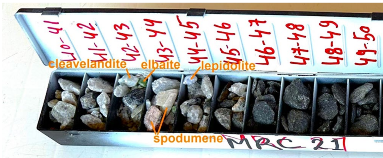
Figure 3: Close-up view of 40m – 50m interval of the 40m-60m chip tray of MRC21.
