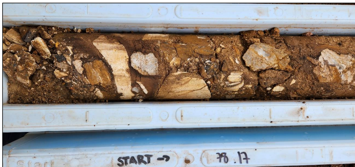
MLJDD020_178.0m_Polymictic Breccia with silica-pyrite clast
