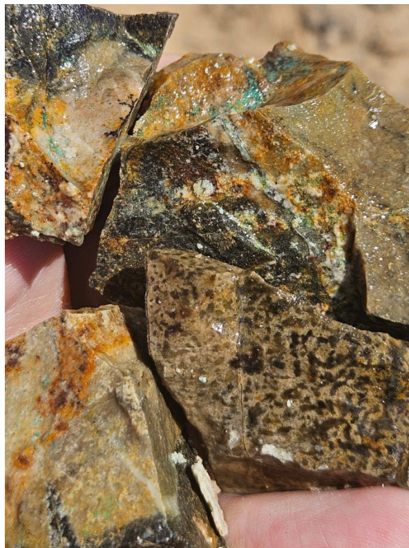
Figure 4: Hornfels, some with secondary biotite, with green and black copper oxides in fractures associated with quartz. Multiple generations of fine quartz veining indicate more than two hydrothermal events (262100E, 8060641N). 1
