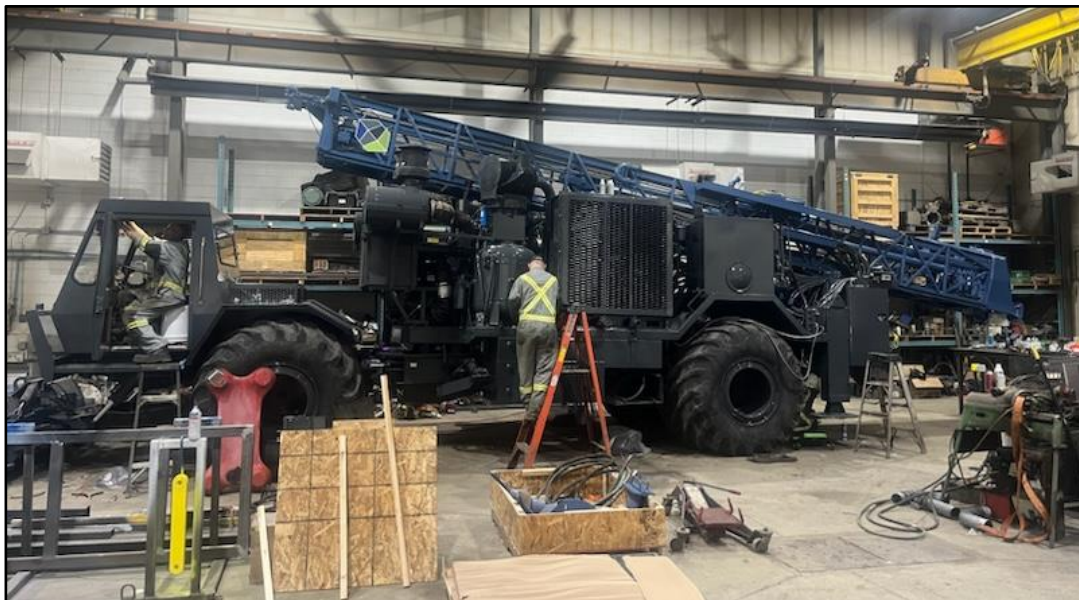
Figure 2. Workshop re-assembly of the Reverse-Circulation drill rig ahead of its mobilization to Red Mountain.
