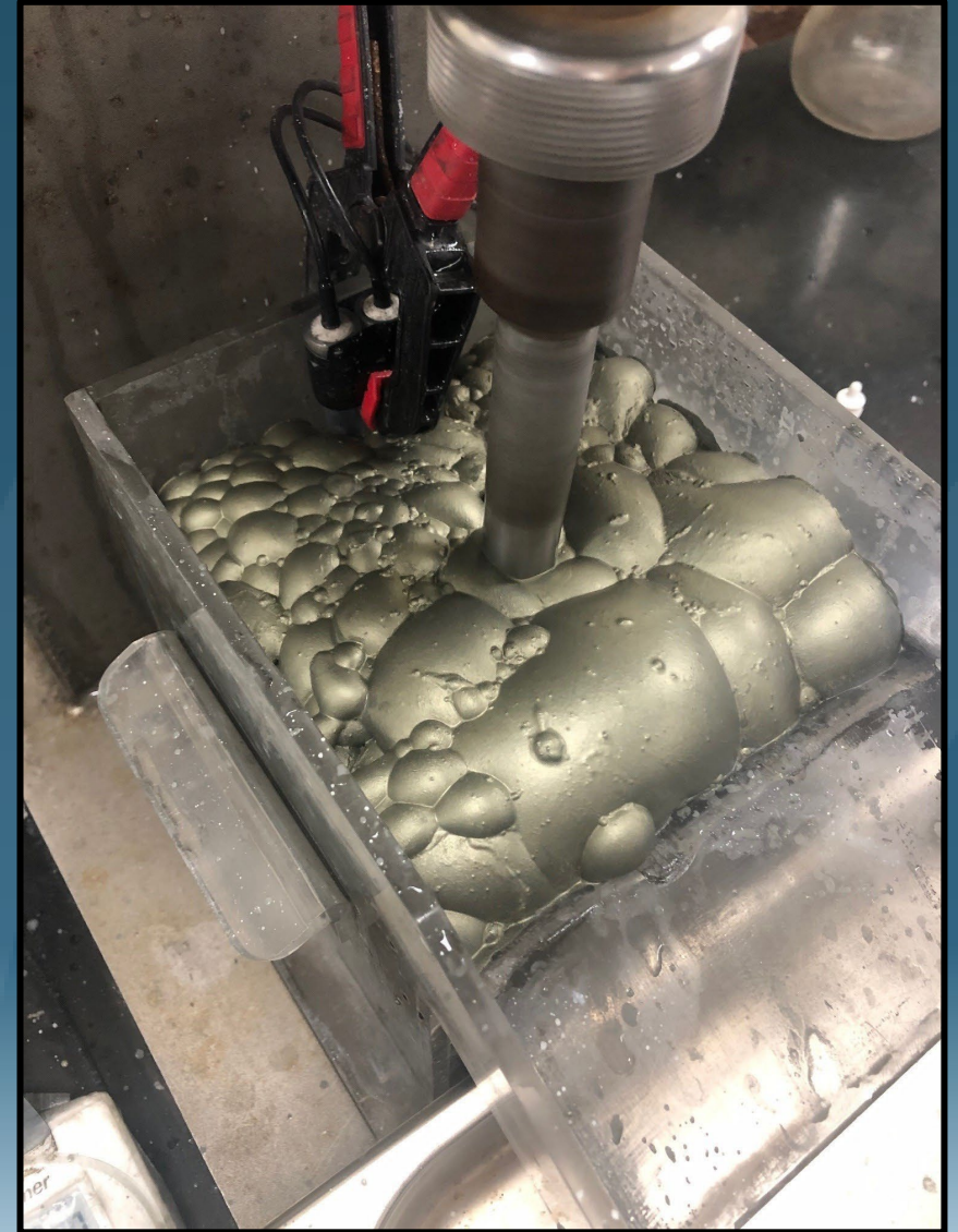
Sulphide flotation of Callisto sample from NRCD337
