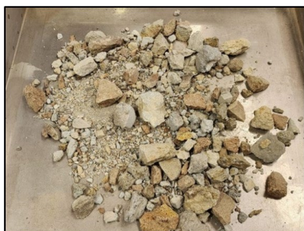
Figure 11: Medium Grade Sample Prior to Scrubbing
