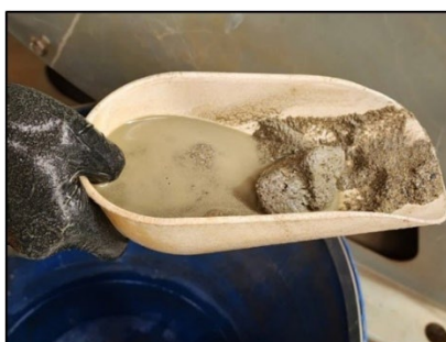
Figure 13: Sample taken directly from the scrubber showing coarser lumps and middlings, sand-like particles
